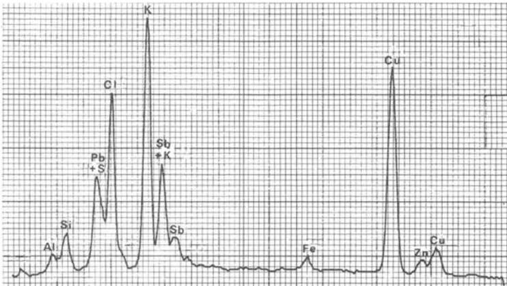
FIG. 15—Spectrum for 9-mm Israeli ammunition fired by Uzi submachine gun at range of 50 m.
