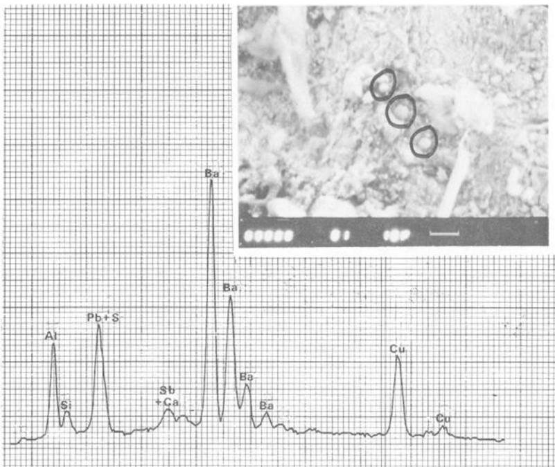
FIG. 2—A 9-mm Israeli bullet fired by Uzi submachine gun at a range of 25 m. Photograph shows spherical primer particles on bullet's core. Spectrum is for the middle particle.
