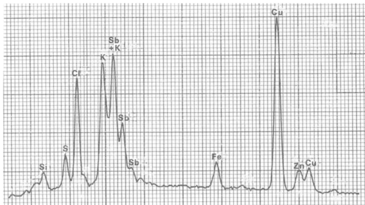
FIG. 14—Spectrum for 7.62 armor-piercing incendiary ammunition (Egyptian) fired by Kalishnikov rifle at range of 50 m.
