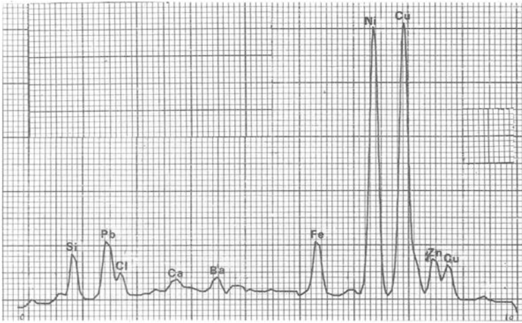
FIG. 4—Spectrum for Hirtenburg 9-mm short ammunition fired by Beretta pistol at range of 25 m.
